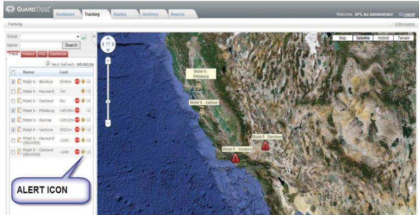
By clicking on the TRACKING tab at the top of the GuardTrax web site, a list of devices can be seen in the column on the left of the screen. To the right of the device name, there is a yellow diamond icon. By clicking on this icon, an information box will appear displaying Events, Alerts, and other important information.
